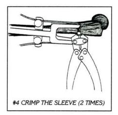
4. CRIMPING THE SLEEVE: Insert the jaws of the crimping tool over the center of the sleeve and crimp. This should be done two (2) times to insure a tight interface between the sleeve and the cable. After crimping, inspect to assure a tight lock.
