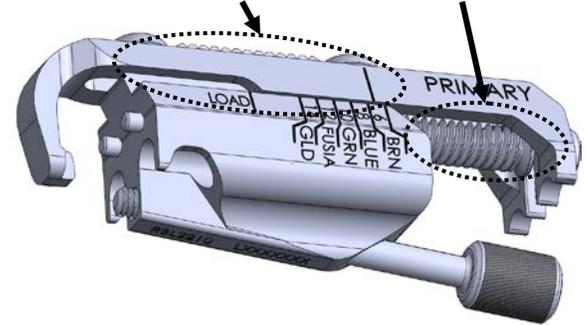
**Figure 4 – Low-Profile Primary Guide Lubricant Application Area**
