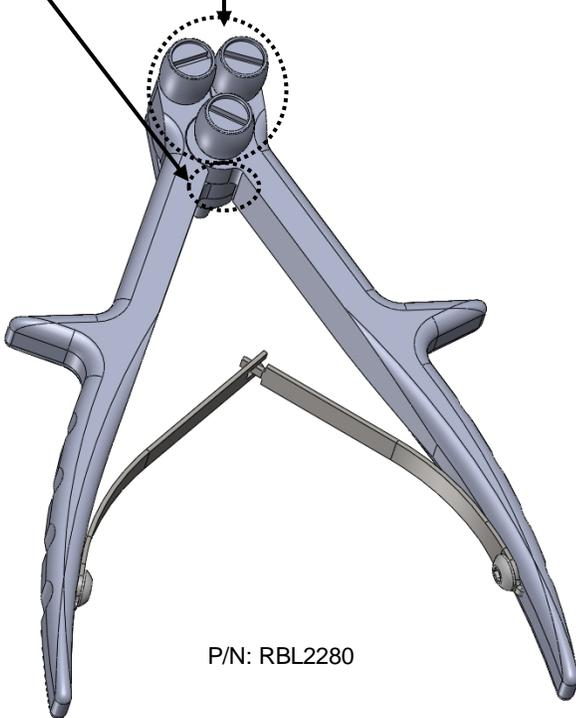
**Figure 2 – Intermediate Gauge Lubricant Application Areas**
