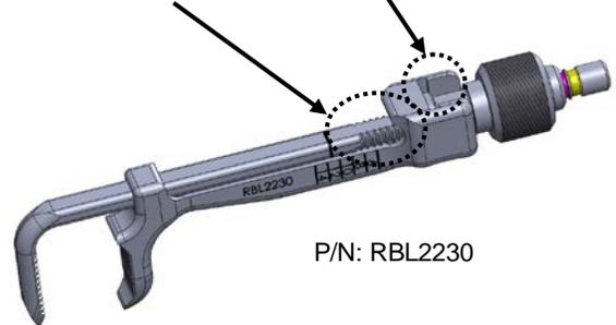
**Figure 3 – Primary Guide Lubricant Application Areas**
