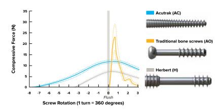
The above graph illustrates the window of screw rotations during which each screw delivers maximum compressive force. The Acutrak screw has the largest window of compression, which is attributed to the additive property of each variable thread pitch providing compression on the fully threaded screw.
