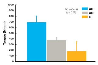
Acutrak® screws have the highest resistance to torsional loading when compared to AO & Herbert bone screws (AC) $^9$
