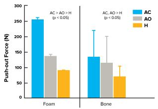
Acutrak® screws have the highest push-out force when compared to AO & Herbert bone screws (AC) $^{9}$
