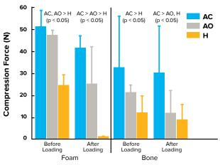
Acutrak® screws have the highest amount of retained compression after cyclic loading when compared to AO & Herbert bone screws (AC)<sup>9</sup>
