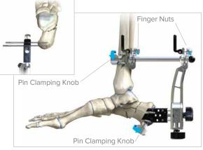
PULL FRACTURE OUT TO LENGTH Using the Cal-Jak for leverage, reduce the tuberosity and pull the fracture out to length. Close the Cam-levers down to lock the positioning of the calcaneus. Additional fine tune adjustments can be made using the Fine Adjustment Knobs.
